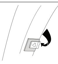
Wrap Black Mylar Tab over hole, then install U-Clip on top of it.
