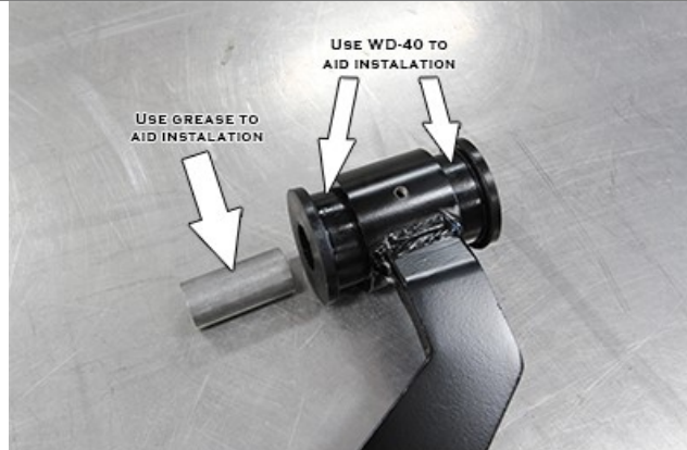
Figure 3: bushing and crush sleeve installation
