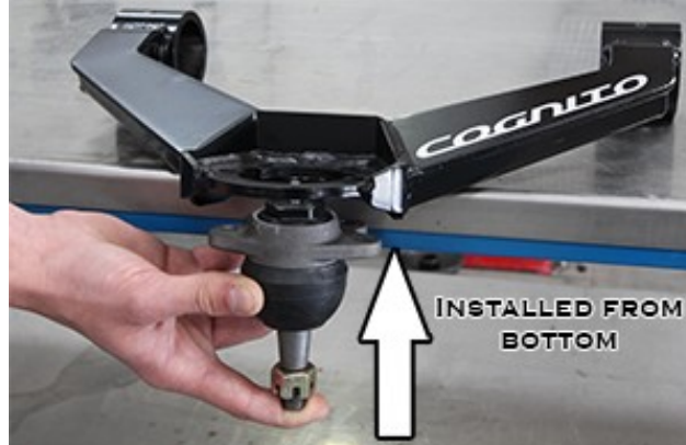
Figure 2: ball joint installation
