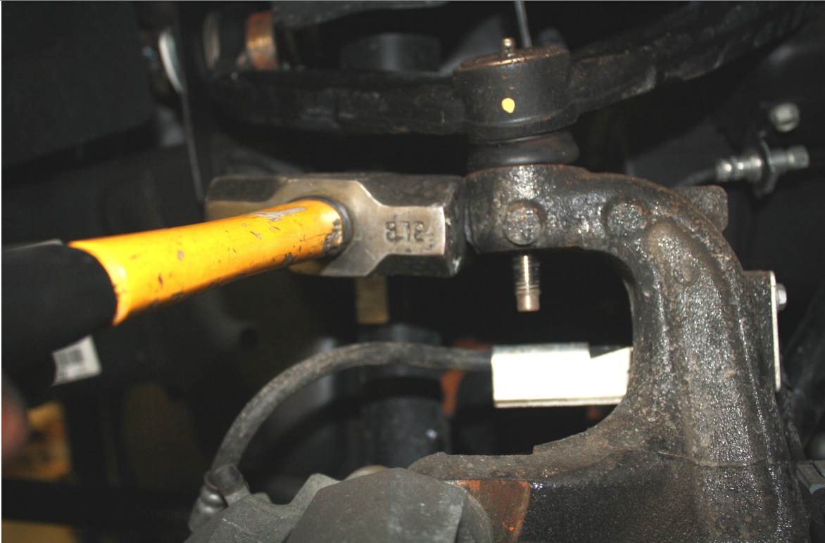
Figure 1: breaking ball joint loose from spindle
