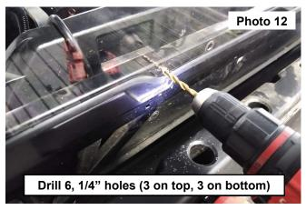
12. Drill 6, 1/4" holes through the windshield into the metal frame (3 on top and 3 on bottom of windshield). **See Photo 12 and 14**.
