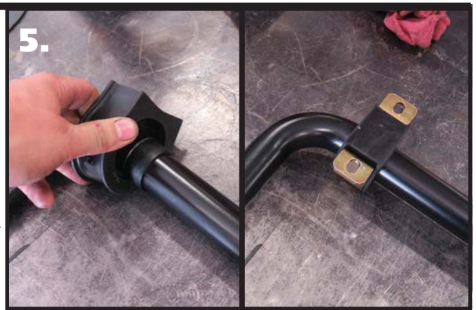
5. Open the SwayBar Bushing at the split and slide it OVER the Delrin Liner. Do this on both Delrin Liners. Next, slip the Bushing Straps over the SwayBar Bushings.
