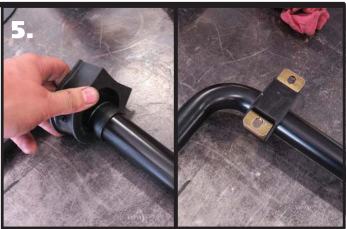
5. Open the SwayBar Bushing at the split and slide it OVER the Delrin Liner. Do this on both Delrin Liners. Next, slip the Bushing Straps over the SwayBar Bushings.
