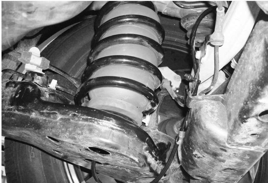
Inside, forward of axle view of passenger's (right) side installation
