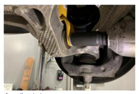
12. Swing the control arm down and away from the strut.
