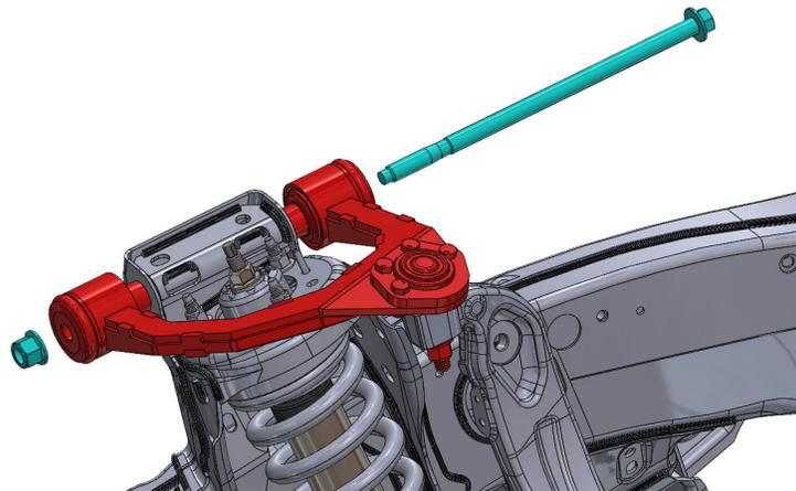
10. While holding the arm up so the top of the ball joint sits level to the ground, torque the mounting bolt to oe spec.
