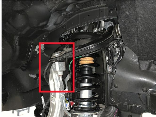
11. Use a puller tool or strike the spindle with a hammer to separate the ball joint from the spindle.
