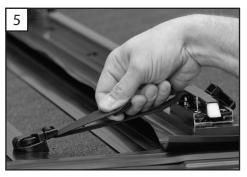
3, 4 & 5. Release the strap from the stowed position by squeezing the tabs. Attach the buckle at the bulkhead, pull the strap to take up the slack and secure the cover. Repeat this for the opposite side.
