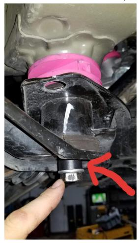
a. Re-install main subframe bolts 2 turns. Allowing the subframe to drop will give you enough space to put the strut back in - it will be 2" longer than
