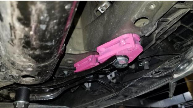
28. Install subframe bracket spacer 33.20 at rear corners of subframe. Tab with hole in it should be away from the body.
