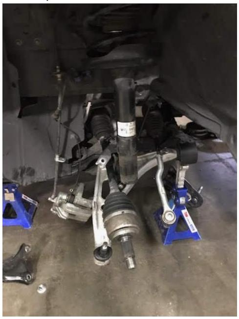
9. Remove bolt on passenger side lower control arm and install washer to increase the clearance between the bolt and the axle shaft. OPTION - grind bolt threads
