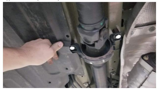
37. Install skid plate tube frame drop spacers, using supplied bolts.
