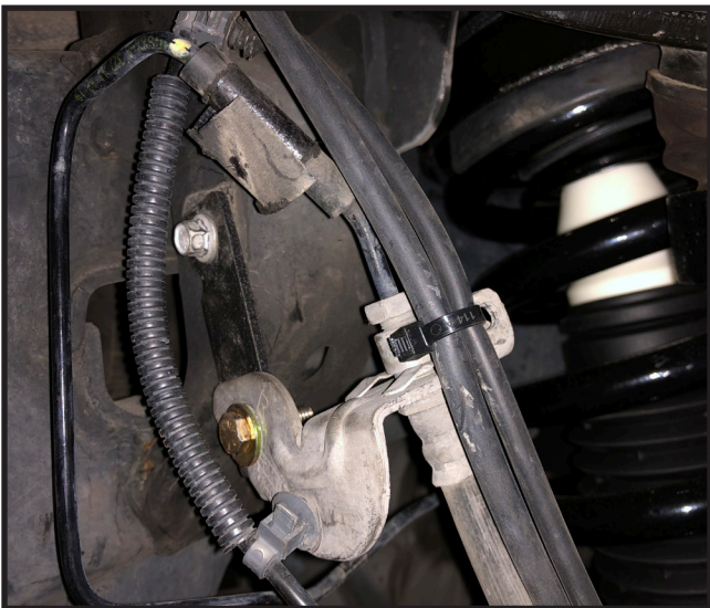
64. Re-install the outer tie rods into the new steering knuckles.
