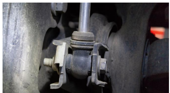
Figure 16B: Front Lower Shock Mount Installed
