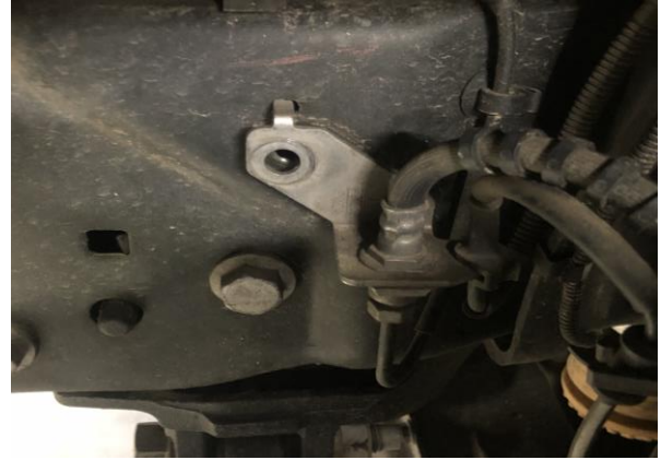
Figure 1B: OE Brake Line Bracket, Bolt Removed
