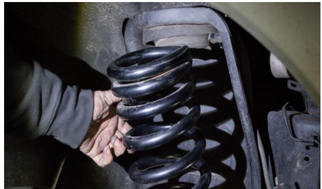
Figure 9B: Spring Removal
