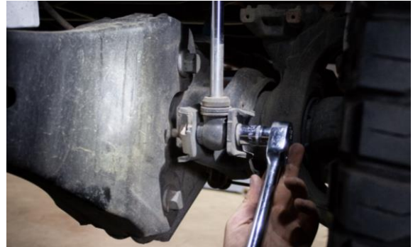
Figure 8B: Front Shock, Lower Mount
