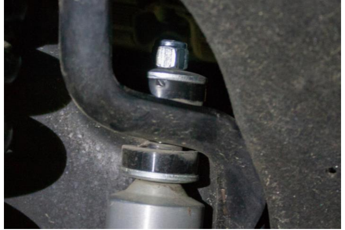
Figure 15B: Top Shock Mount Installed
