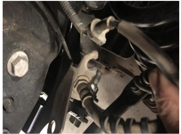
Figure 2B: Driver ABS Line Removal
