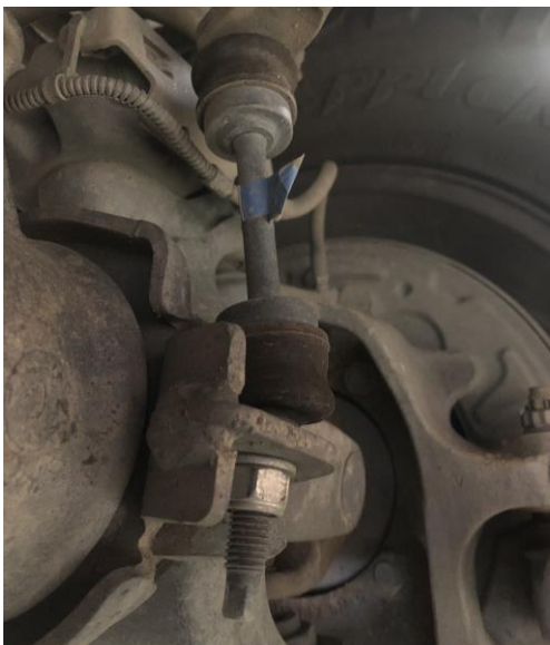
Figure 7A: OE Sway-Bar End Link
