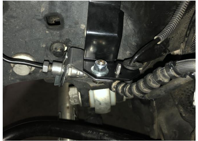
Figure 6: Passenger Side ABS Line Routing
