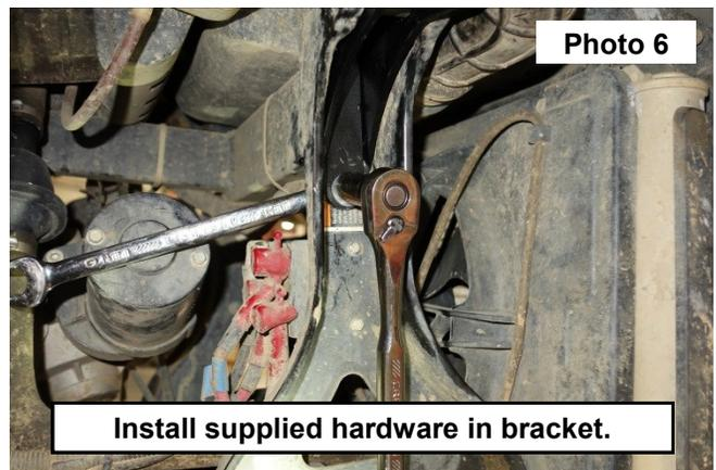
6. Reinstall strut in bracket using stock hardware.
