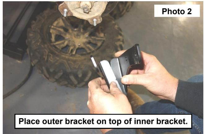
3. Place the outer bracket on top of inner bracket (Photos a and b from page 2) and install in the stock upper strut location using 10mm x 55mm bolts and 3/4" x 0.9" spacer sleeve using two 17mm socket/wrenches. **See Photo 2, Photo 3, and Photo 4.**
