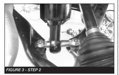
3. Measure 6-1/2" from the coil bucket on the frame and mark the first hole for the resi mount. Then, use the resi mount to mark the second hole. Using a 1/4" drill bit, drill both holes.
