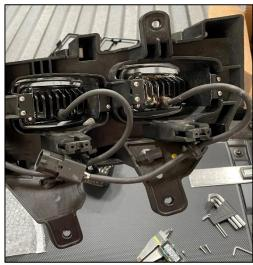
5. Using the supplied wire harness adapter, connect the adapter to the light and OEM wiring. The same functions will power the lights...
