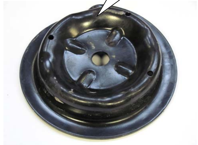
Stahlfederteller Steel spring perch.
