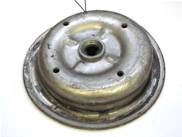
Aluminiumfederteller Aluminum spring perch.
