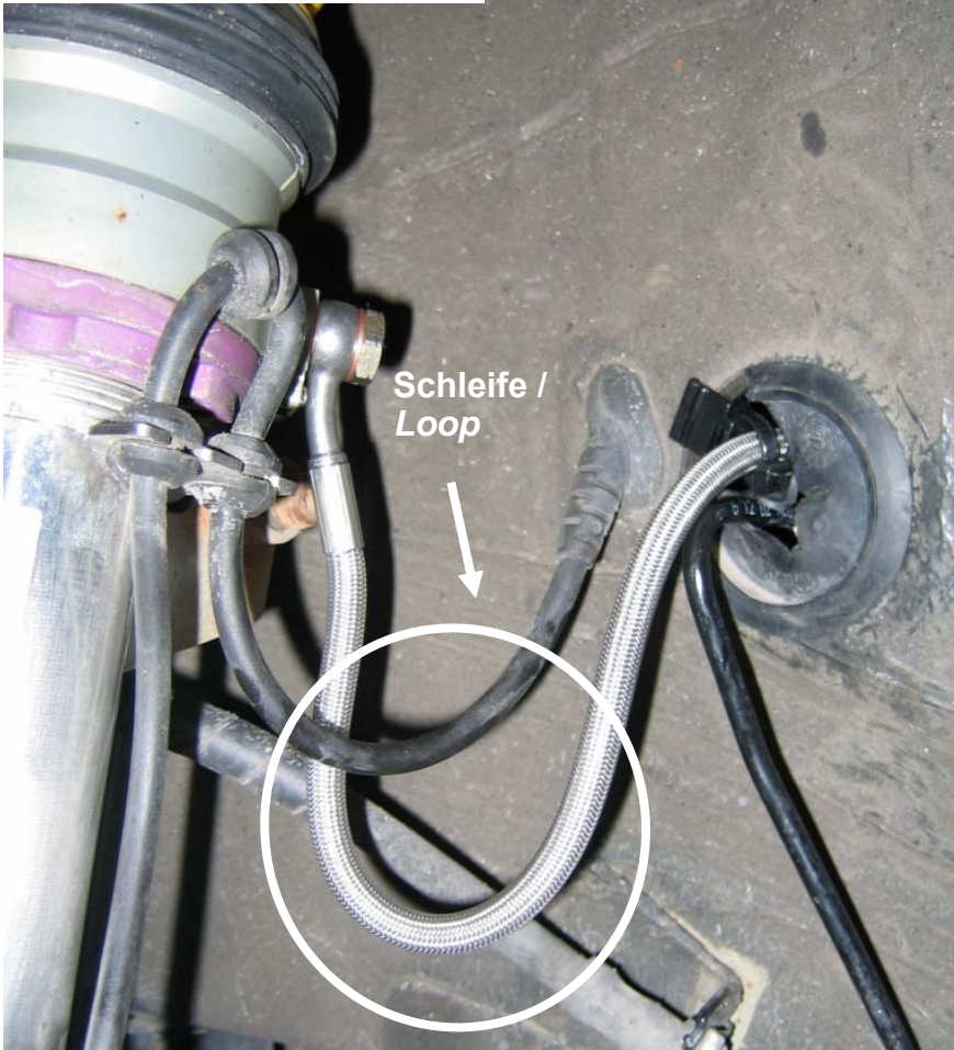
Montageposition 2 / Assembly position 2
