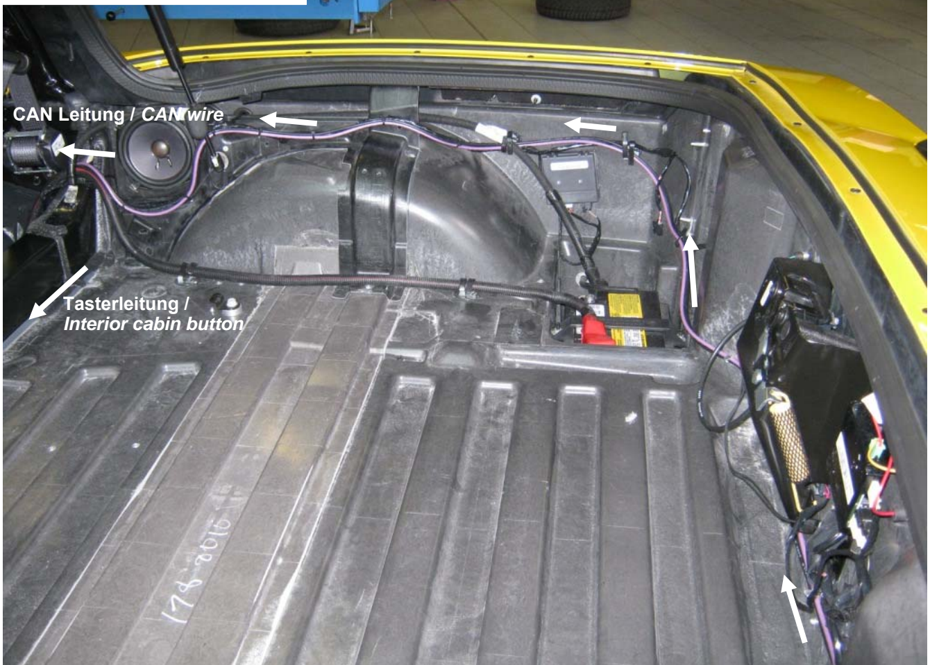
Montageposition 3 / Assembly position 3
