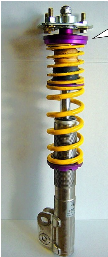
Komplett angeliefertes KW Federbein. Completely pre-assembled KW coilover strut.
