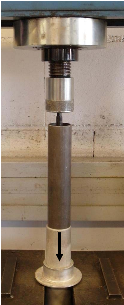
Zerlegtes Federbein ohne Federteller. Disassembled strut without spring perch.
