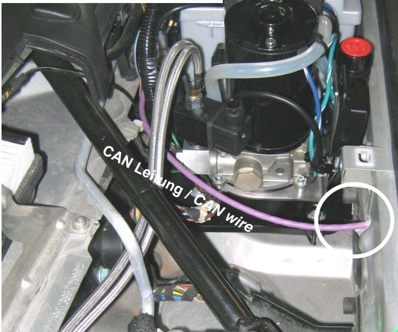
Montageposition 7 / Assembly position 7
