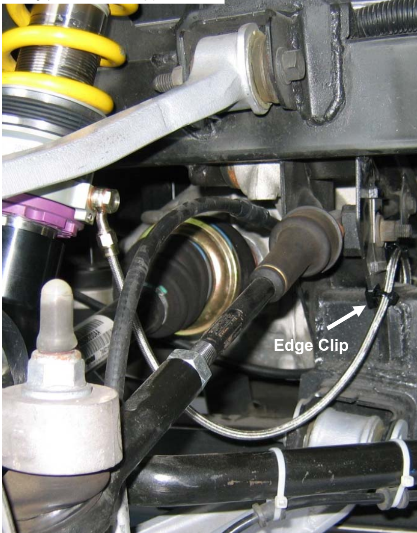
Montageposition 9 / Assembly position 9
