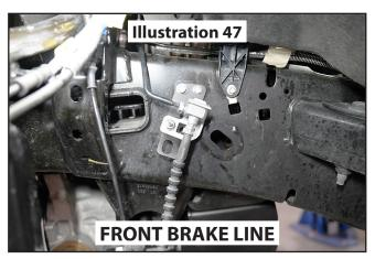
84. Locate the new brake line brackets (55-13-9955 driver, 55-14-9955 passenger) and the supplied 1/4" self-tapping bolt; thread the self tapping bolt into the top 1/4" hole in the bracket (the self tapping bolt is just acting as a locator pin). [7/16"]
