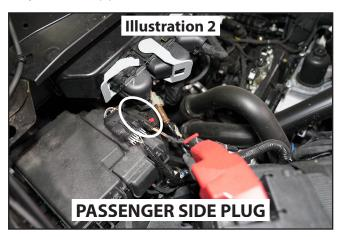
5. Once unplugged, the wires will need to be unclipped and from the retainers and pulled out toward the knuckle to allow the knuckle assembly to be removed from the vehicle in a later step.
