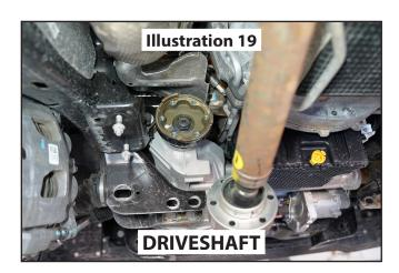
20. Secure the driveshaft up and out of the way.
