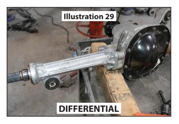
39. Apply the supplied RTV gasket maker to the axle housing, making sure there are no gaps of RTV in the application.
