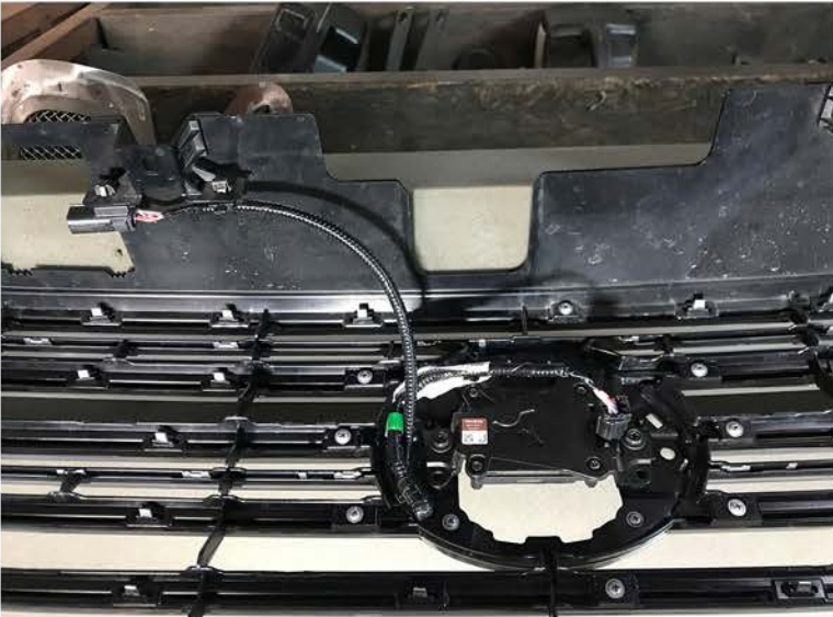
3. Remove TSS sensor module and harness from factory grille. Note the TOP side orientation of the sensor.
