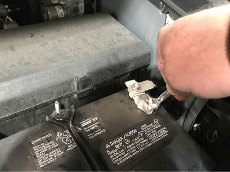
1. Disconnect negative battery terminal.
