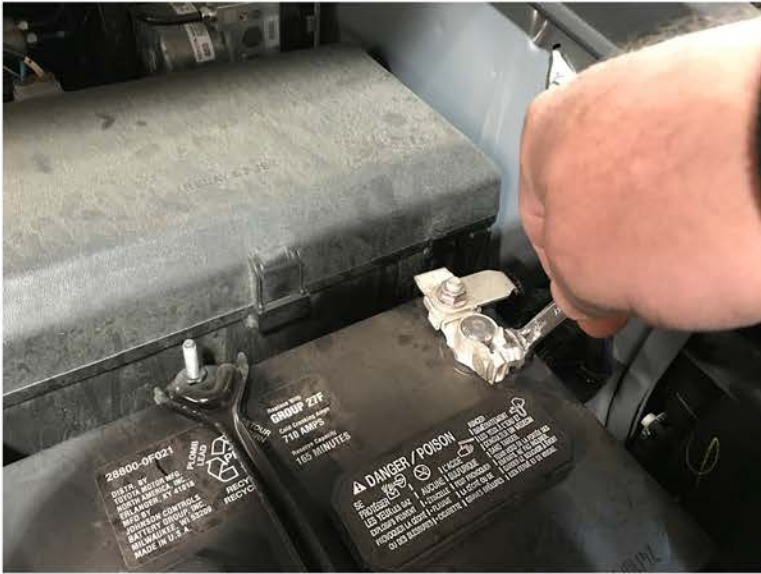
1. Disconnect negative battery terminal.
