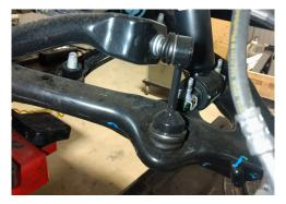
12. Push or pry down on the lower control arm to gain clearance and remove the strut.
