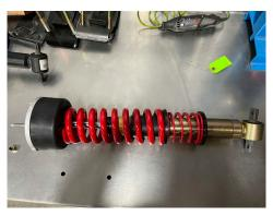
25. Reference the OE strut markings and ensure the top mount is oriented in the same fashion it was before disassembly. Torque the supplied nyloc nut onto the strut to 37 ft lbs.
