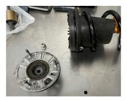
16. Remove the spring and strut from the fixture.
