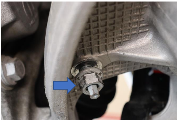
Step 8. On both sides, remove the front stabilizer link lower nut from the lower control arms.
