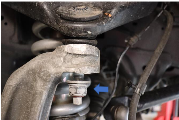
Step 22. Use a pry bar to ease the upper control arm down into the spindle and fasten the nut on the bottom. Torque nut to 26 Ft. Lbs. + 180°
