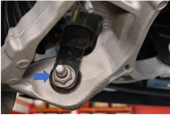
Step 19b. (Torque nut to 124 Ft. Lbs.)
