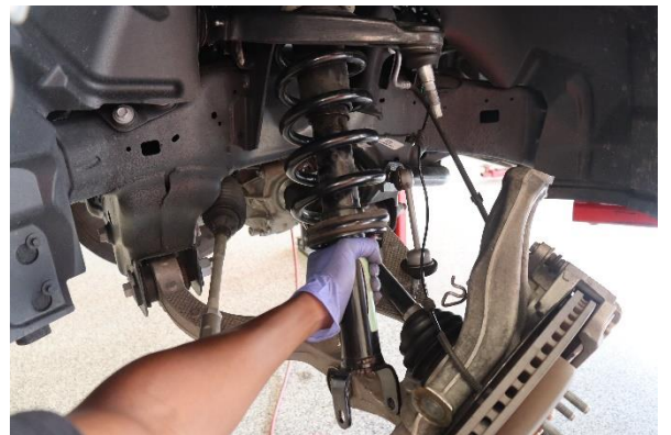
Step 14b. Note: Ensure knuckle does not pull on brake line, or that it is not pulling on the axle. Tie strap the knuckle to frame if necessary.
