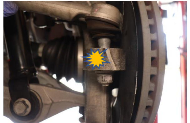
Step 7. Shock with hammer until it separates. Remove the tie-rod nut and set the tie-rod aside.
