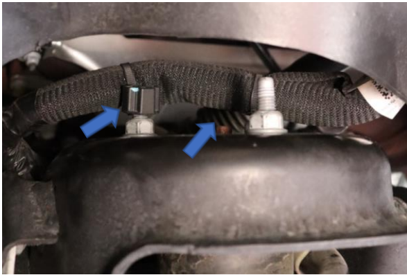
Step 12. Separate the wire harness from the strut assembly studs.
