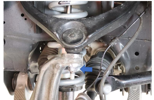
Step 22b. (Torque nut to 26 Ft. Lbs. + 180°)
