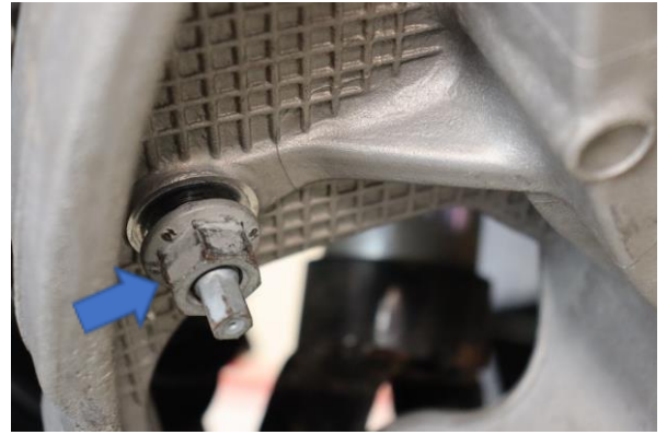
Step 20. Re-insert the stabilizer bar end link and secure the nut at the bottom. Torque nut to 88 Ft. Lbs.
