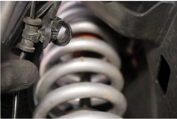
Step 24. Reattach the speed sensor wire to the upper control arm bracket.
