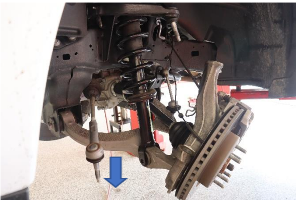
Step 14. Press downward on the lower control arm and remove the strut assembly.
