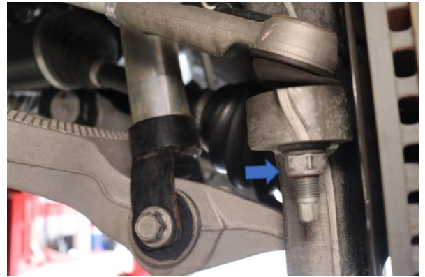
Step 21b. (Torque nut to 38 Ft. Lbs. + 195°)
