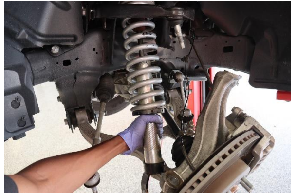
Step 16. Install new Eibach Coil Over shock
