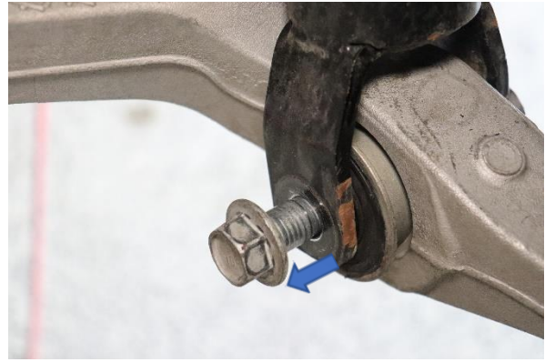
Step 11. Remove the shock assembly lower bolt.
