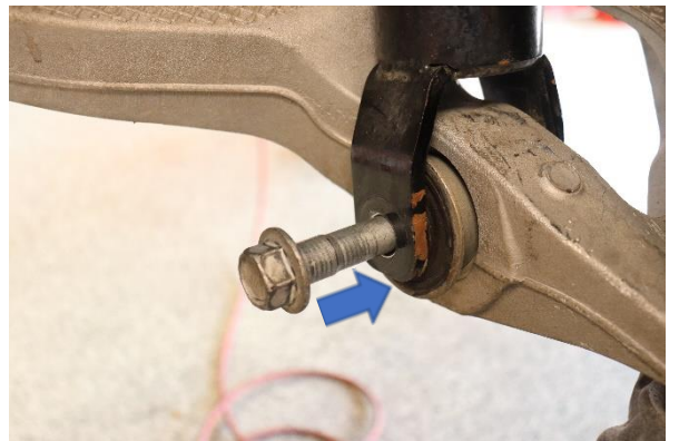
Step 19. Reinsert the lower shock bolt and secure the nut. Torque nut to 124 Ft. Lbs.
