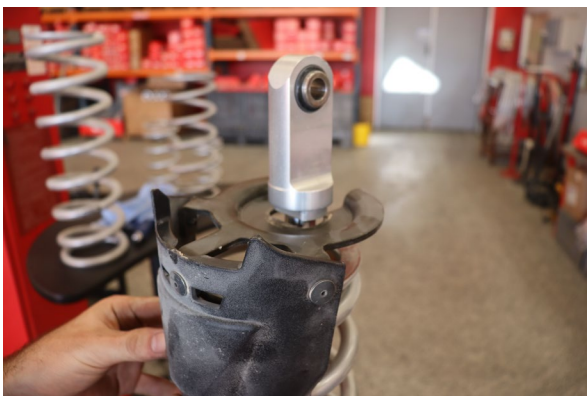
Compress the springs and install the OE lower spring perch. Make sure to align the boss on the rod end as shown.
