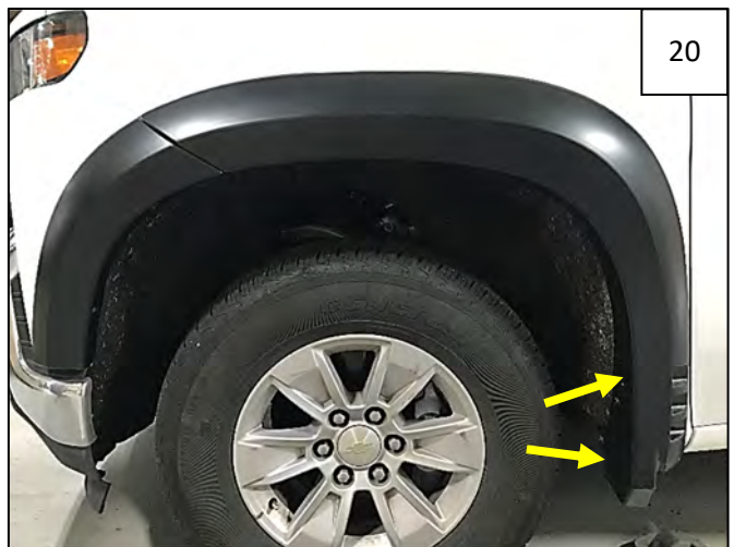
Start 2 factory T15 Torx screws at bottom rear of wheel well as shown. Apply pressure to outward face of the flare towards the center of the vehicle and tighten all screws.
