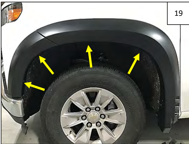
Align flare on vehicle and start 4 supplied Truss-Head Screws through holes in flare and into fender as shown.
