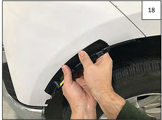
Use thumbs to fully press tape against vehicle, working along part.
