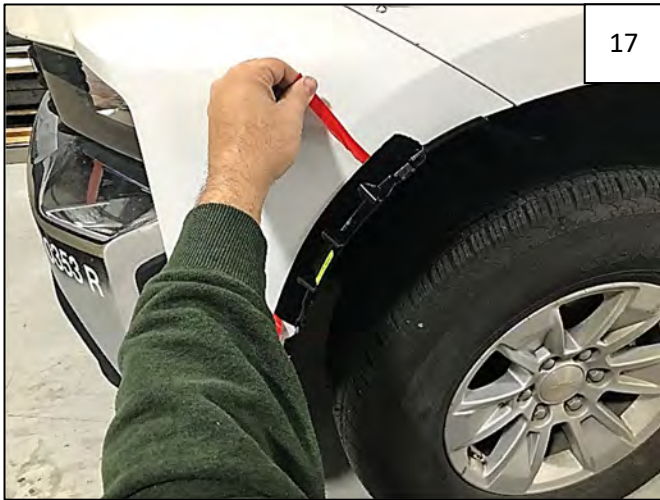
Pull leader from upper tape on Inner Bracket.
