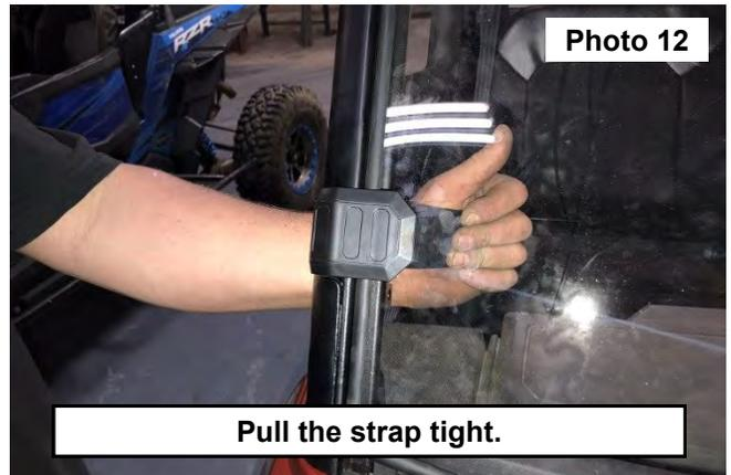
12. Secure by finishing the wrap around the strap. **See Photo 13.**
