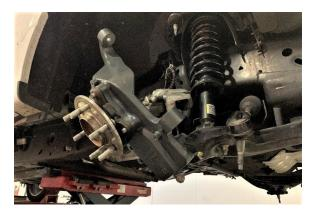
23. Mount the upper ball joint onto the Belltech spindle and secure the upper ball joint nut so it is hand tight, do not torque yet.
