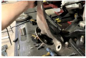
21. Once the spindle has been removed from the vehicle, remove the hub bolts detach the hub from the spindle.
