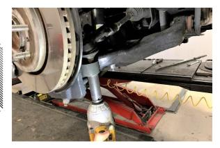
30. Reconnect the upper end link to the spindle. Torque the upper nut to 111 ft lbs.
