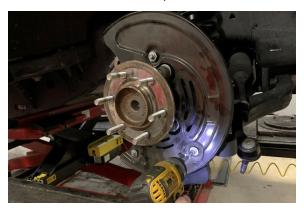
27. Remove the zip tie, wire, or hook that is holding the caliper out of the way. Place the caliper over the rotor and fasten it onto the Belltech spindle using OEM bolts. Torque the caliper anchor plate bolts to 184 ft lbs.
