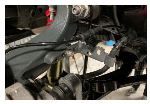
2. Mount the steering tie rod end onto the Belltech spindle and torque to 66 ft lbs.
