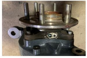
22. Mount the Belltech spindle onto the bottom ball joint and secure the bottom nut so it is hand tight, do not torque yet.
