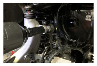
10. Remove the 21mm nut on the steering arm tie rod end. To detach the ball joint from the spindle, carefully strike the boss with a hammer or rubber mallet.
