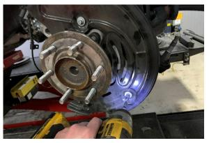
15. Detach the ABS sensor from the hub with a 5mm hex key.
