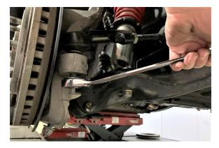
11. Remove the 10mm nut holding the break line bracket to the spindle. Also remove the clips holding the lines to the chassis with a trim removal tool.
