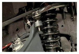
24. Raise the lower control arm with a transmission or floor jack to simulate a load on the suspension. Torque the lower ball joint nut to 98 ft lbs. and the upper ball joint nut to 46 ft lbs.
