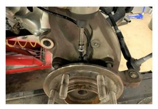
16. Break loose but do not remove the 18mm upper ball joint nut.
