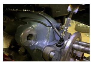
26. Reinstall the OEM dust shield and brake rotor onto the Belltech spindle.
