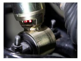
28. Attach the end link to the lower control arm, torque to 74 ft lbs. when the suspension is loaded or the vehicle is back on the ground.
