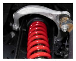
27. Attach the lower strut mount to the lower control arm using the supplied bolts, washers and Nyloc nuts. Torque the supplied nuts to 60 ft lbs.
