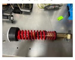
25. Reference the OE strut markings and ensure the top mount is oriented in the same fashion it was before disassembly. Torque the supplied nyloc nut onto the strut to 37 ft lbs.
