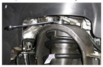
10. Remove the bottom bolts on the OE strut and lower control arm using a 15mm wrench.
