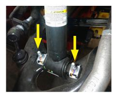
11. Remove the mounting nut holding the anti-sway bar end link to the lower control arm. The nut is located on the underside of the lower control arm. This will allow the lower control arm to swing down and ease the removal of the strut.
