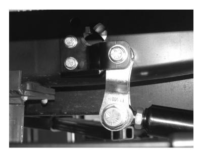
9. Loosen all the jam nuts away from the bars and make sure that the required 1" of thread is in each of the bars (there is 1 ¾" of threads total on the ends). Apply some of the supplied thread locking compound to each joint and retighten the jam nuts. Torque the 3/4" bolts to \*\*450 ft. lbs.
