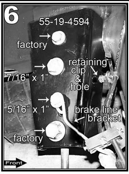
brake line bracket - to - Superlift bracket. Tighten the 7/16" hardware (50). Tighten the 5/16" hardware (200 in. Lbs.). Tighten the factory hardware (top hole) (23).
