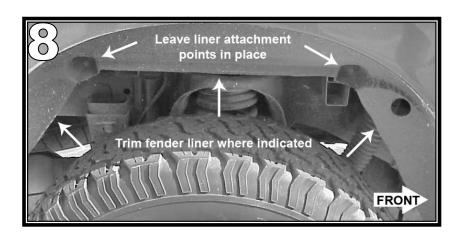
trimmed to minimize contact to the tire. Trim the liner horizontally on the angled face above the area of contact. Leave the two fasteners intact and trim the liner at an angle on each end to meet the bottom of the liner. Paint any exposed surfaces black for best appearance.
