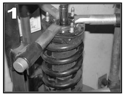
□□ Carefully remove the strut cylinder from the coil spring.
