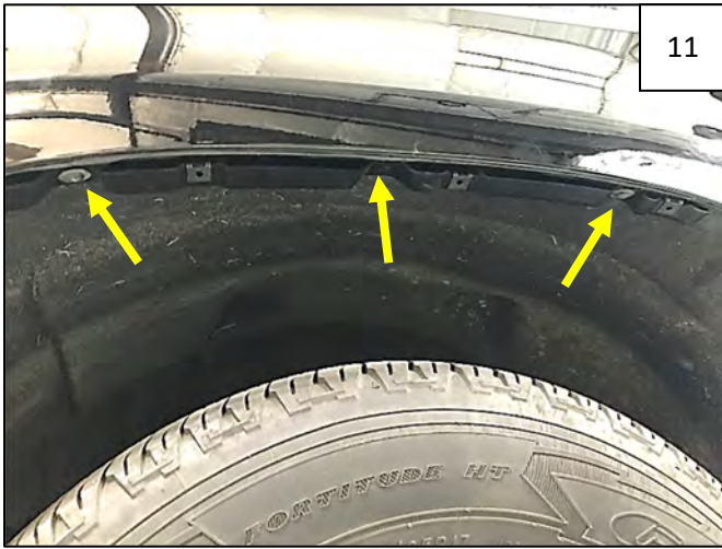
Install Long Inner Piece onto top underside lip of fender using 3 factory screws.
