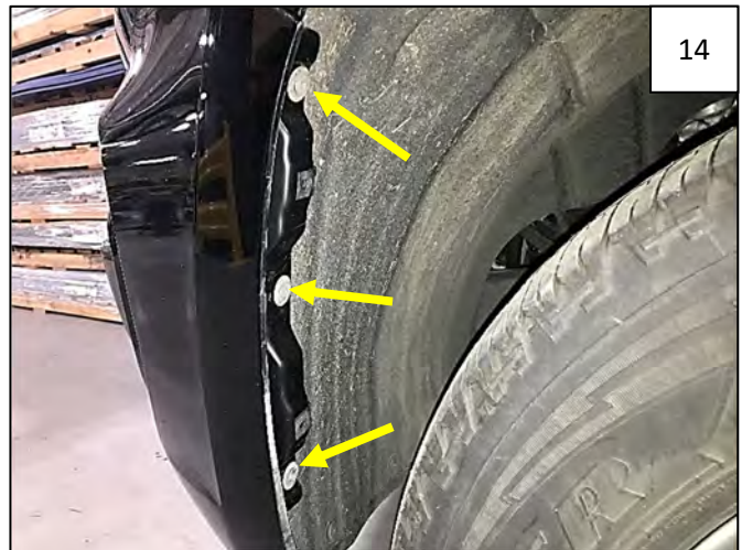
Install Short Inner Piece onto front lip of fender using 3 factory screws.
