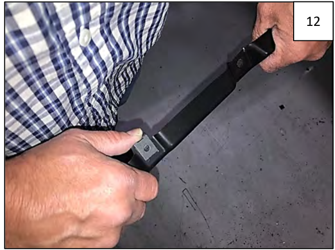
Install 2 supplied Short "U" Clips over holes in Short Inner Piece.
