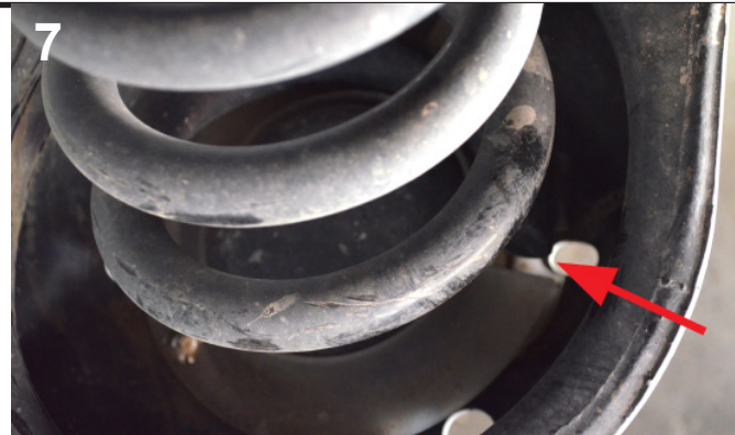
Reinstall coil spring, making sure the bottom of the spring lines up correctly in the LCA, see image.
