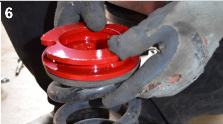
Install the Traxda spring spacer onto the coil spring.
