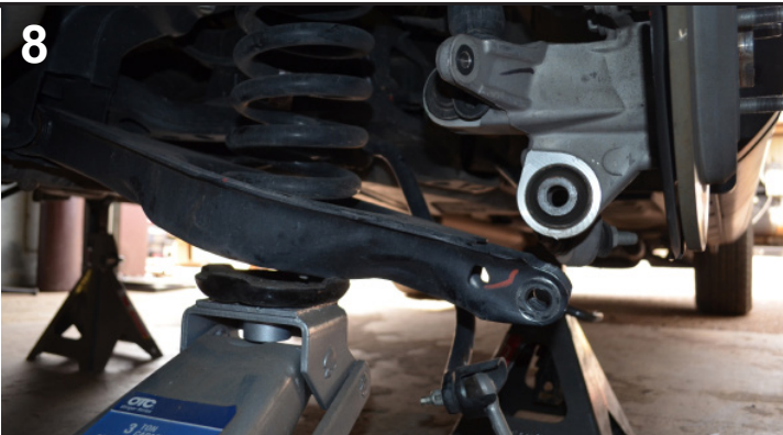
Using floor jack apply pressure to LCA until it lines up with knuckle and replace bolt. Do not tighten LCA until vehicle is back on ground.
