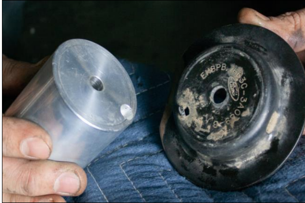
Figure 6: Bump Stop Spacer and OEM Mount
