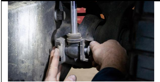
Figure 12: Front Lower Shock Mount
