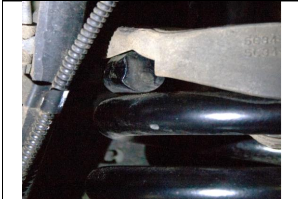
Figure 8: Top Spring Pigtail Installation
