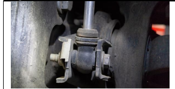
Figure 13: Front Lower Shock Mount Installed
