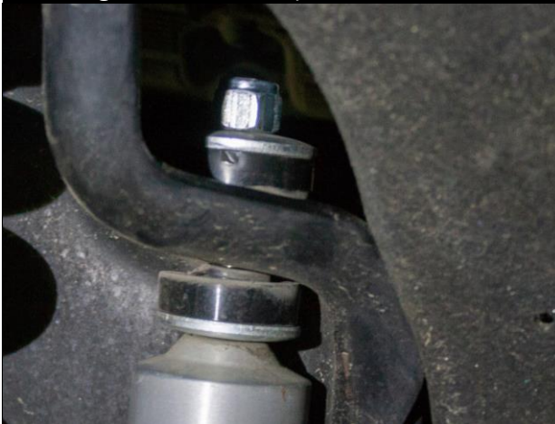
Figure 11: Shock Top Mount Installed
