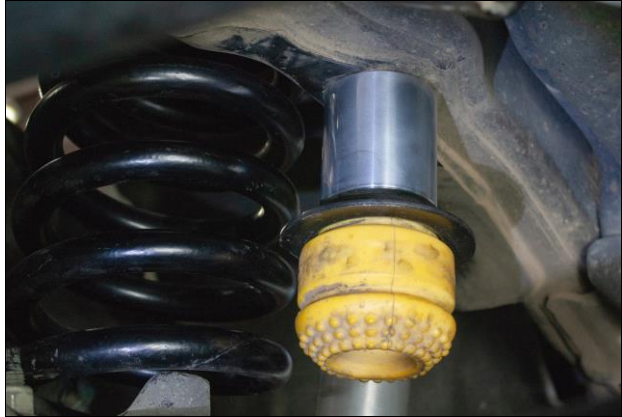
Figure 7: Assembled Bump Stop Installation
