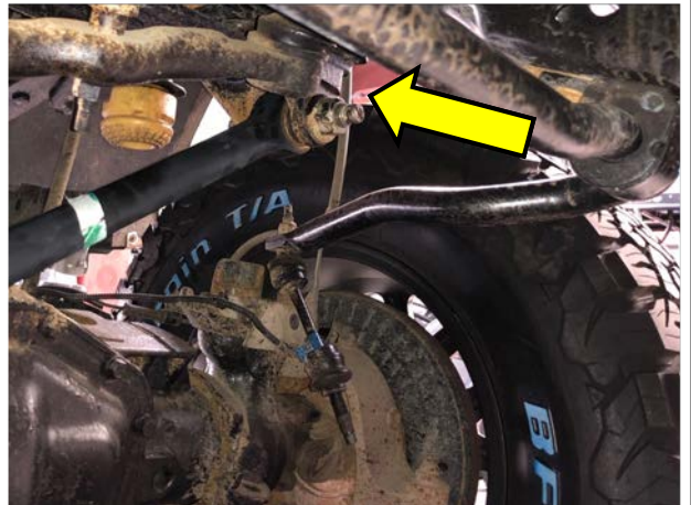
Figure 2: Remove Track Bar to Bracket Nut
