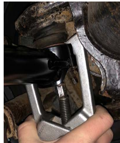
Figure 6: Remove Track Bar with Bearing Puller
