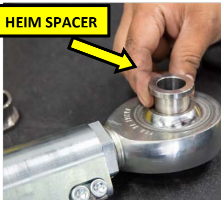
Figure 7: Installing Heim Spacer
