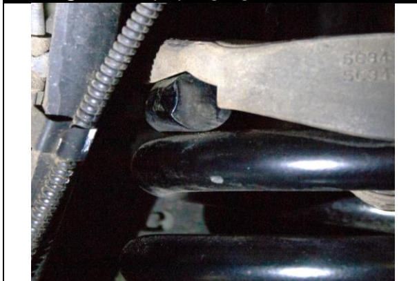
Figure 8: Top Spring Pigtail Installation
