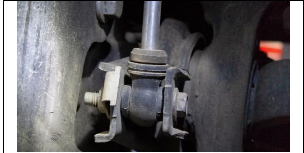
Figure 13: Front Lower Shock Mount Installed
