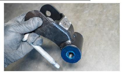
4. Install the shackle onto the leaf springs with the factory bolt and nut, hand tight. The Carli Logo plate will face the rear, the zerk fitting will face the leaf spring. The bolt will install from the INSIDE-OUT. The head of the bolt should face the frame when installed (passenger's side shown). If you flip the bolt, the threads will contact the frame as the shackle moves.
