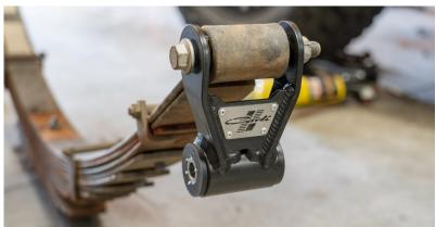
5. Reinstall the leaf springs into the truck and secure with the factory hardware, all hand tight.
