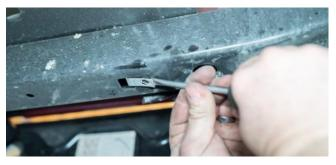
9. 13MM Socket—Remove the 2 bolts holding the upper trim piece to the front of the hitch..
