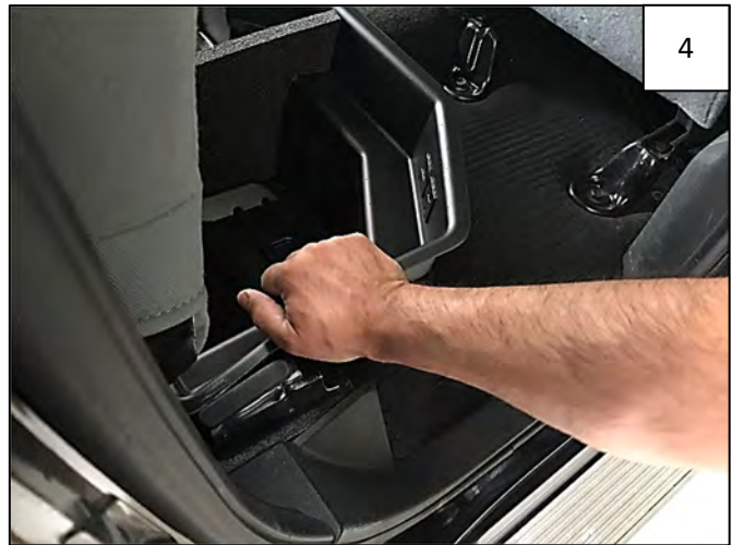
On passenger side, press edge of Underseat Storage Box to seat it underneath the passenger side seat cushion stop.
