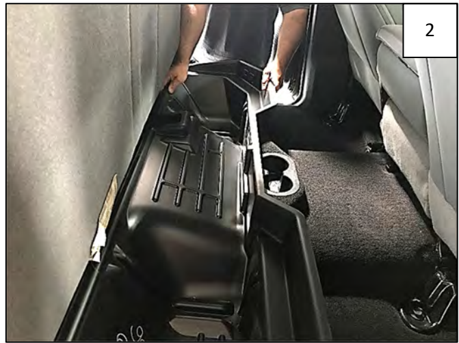
Nest the Underseat Storage Box into factory underseat indent. The driver's side of the Storage Box should slide underneath seat cushion stop as shown in next step.
