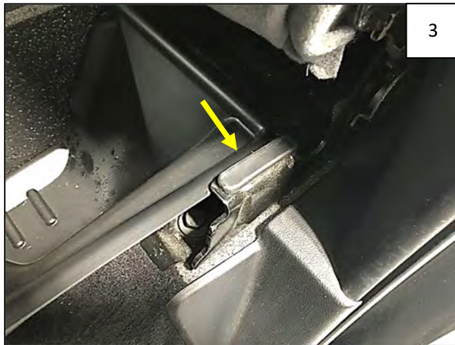
Make sure the driver side edge of Underseat Storage Box is guided under seat cushion stop.
