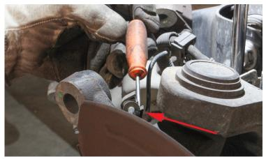
8. 5MM Allen - GENTLY Remove the ABS Sensor from the hub
