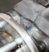
9. 21MM - Remove Drag Link and Tie-Rod from Passenger's side knuckle connection points. We back these nuts off until they're only engaged a few threads then strike the knuckle housing - see arrows below - (NOT the tie-rods) with a hammer under the joint drops. Then remove the nut and linkage.
