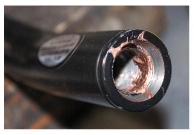
6. Thread the provided jam nut all the way to the end of the shank on the heim-joint so it's tight against the housing. Thread the heim joint 1-2 threads into the track bar. Apply RED LOCTITE to **ALL** the exposed threads of the track bar. These are the threads on which the Tapered-Jam Nut will sit.
