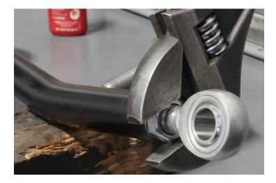
12. Confirm ends remained parallel during torquing. NOTE: Note the position of the jam nut. The flat part of the "hex" on the jam nut is indexed so it is parallel to the rod-end's orientation. This will ensure that the jam nut does not rub the factory track bar pocket. If the "point" of the jam nut faces the rear of the track bar, the jam nut will rub the bracket and could loosen.
