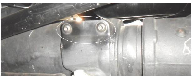
3. Use the provided  $\frac{1}{2}$ " button head bolt to replace the factory axle side steering stabilizer bolt. Ensure the nut faces the ground and torque to 35 ft.lbs.
