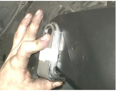
**19.** Use a ½" Drill bit to slide into the tool/indexed crush sleeve and drill the opposing side of the frame rail. **Note:** A right-angle drill will be necessary here.
