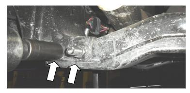
**8.** Using a Plastic Fastener Removal Tool (Christmas Tree), pull the DEF Harness connection out of the Frame and Transmission Crossmember connections to make room for the Radius Arm Drop Brackets.
