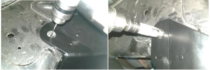
18. Slide the 3/4" OD Crush Sleeve into the provided tool (L-Bracket). Once it's pressed in and centered, slide the 3/4" crush sleeve into the upper, rear frame hole that you just drilled. The L-Bracket will index off the drop. With the tool inserted, clamp it in place to ensure it remains flat during drilling.
