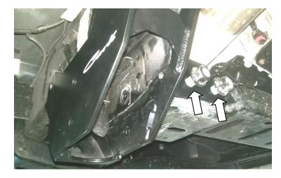
12. Position upper, front, 1" OD Crush Sleeve into the front Radius Arm bracket hole (not through the frame yet), slide the "Q-Shaped" frame spacer between the frame and drop bracket, then slide the crush sleeve through the spacer into the factory frame hole.
