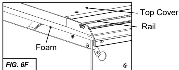
Next mark where the front of the rails sit and mark this position with masking tape, this will be a guide for placing your foam. (FIG 6D). Now pull the cover back until there is room to apply the foam. Lay the foam on the front sill of the truck from rail to rail, trimming the excess with a utility knife (FIG 6E).
