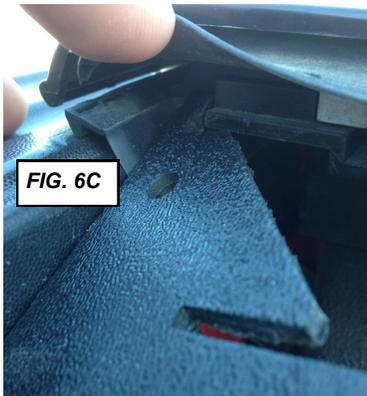
Another way to set the tailgate cap seals is to use the Tailgate Seal Gauge as shown in figure 6B & 6C. You should be able to just slide the Tailgate Seal Gauge in between the Tailgate Cap Seal and the Bottom Cap.
