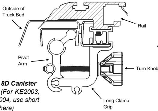
FIG. 8D Canister End (For KE2003, KE2004, use short grip here)
