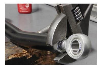
10. Confirm ends remained parallel during torquing. NOTE: Note the position of the jam nut. The flat part of the "hex" on the jam nut is indexed so it is parallel to the rod-end's orientation. This will ensure that the jam nut does not rub the factory track bar pocket. If the "point" of the jam nut faces the rear of the track bar, the jam nut will rub the bracket and could loosen.
