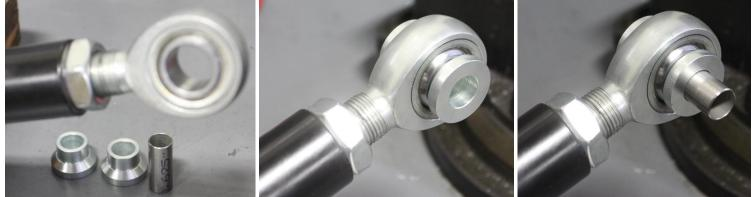
**14.** Slide the assembled heim joint with misalignment spacers (and reducer where applicable) into the axle pocket and assemble with the factory hardware to be torqued later.
