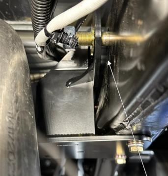
8. If your truck is equipped with the factory 5th wheel hitch, insert the factory 16mm hardware back through the frame rail (and upper airbag bracket—and spacer if utilized) and loosely install the capture nuts on the bolts securing the upper brackets to the frame.
