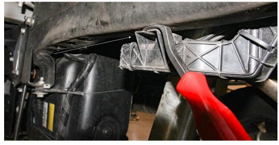
6. Slide the provided captured-nut bracket into the frame in place of the studs that were removed (that retained the factory rear bump stops).
