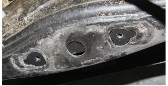
7. Place the Upper bracket into place on the **INSIDE** of the frame rail and use the provided (qty. 2) 3/8"-16 x 1.25" bolts, split lock washers and flat washers to loosely secure the upper bracket to the capture nut bracket inserted into the frame in the factory bump-stop location.
