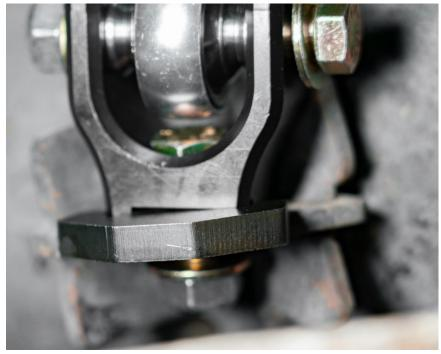
37. Pull Sway Bar down onto the top of the Carli End Link and thread the nut on a few threads.
