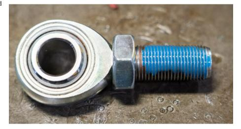
27. Thread the end link back into the body until it bottoms out, then back off until the rod end is parallel with the zerk fitting on the body. 28. Use (2) 15/16" wrenches, one on the body flats, one on the jam-nut, to tighten the jam nut securing the heim's orientation. Use 15/16: Crow's-Foot to Torque jam-nut to 30/ft.
