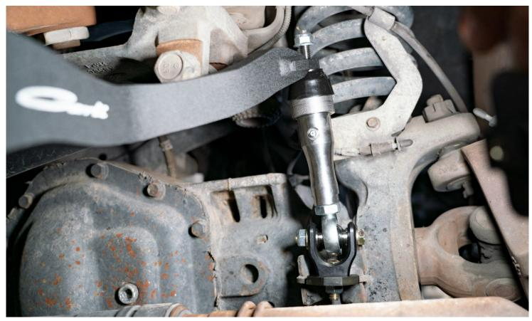
38. Use a 5/16" wrench to hold the hex and 11/16" ratcheting wrench to tighten the sway bar end link nuts to the sway bar arms. The Zerk fittings should be indexed forward for easy access.
