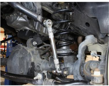
10. From the outside - in, The upper will be arranged: Sway Bar Link, Sway Bar, Flange Nut. **Torque to 75lb.ft.**
